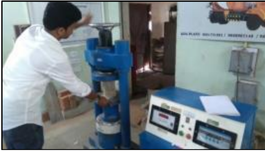
Fig 17 Placing the concrete core of existing RCC raft
