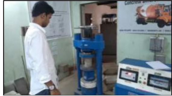
Fig 19 Maximum loading on the concrete core
