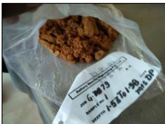
Fig 15 Extracted soil sample at the depth of 1.53-1.98 mt
