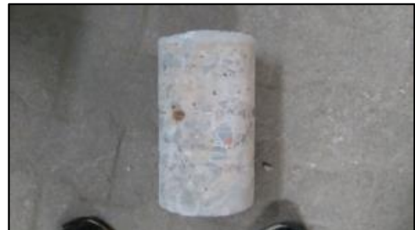
Fig 8 Concrete core from existing raft slab
