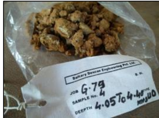
Fig 16 Extracted soil sample at the depth of 4.05-4.40 mt
